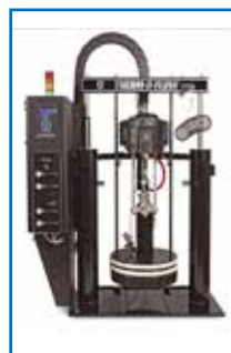
Ensemble de pompage à chaud 200l Heated equipment 200 liters
